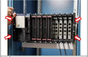
When all BLK connectors are removed from the rack, 5 unsecure the rack using the screws and remove it.
