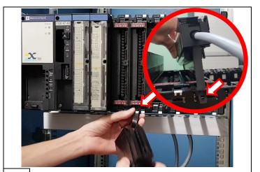
Extract the securing tabs by pressing the inner clips to fully disengage the terminal block from the TSX rack.
