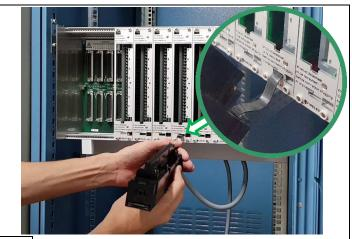
Insert the securing tabs fir each ADP-TSX into the intended slot.
