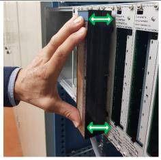
Place the BLK connector and hold it in place with the screw being in contact with the adapter faceplate. Be sure to verify the correct alignment. Don't push it, it will be secured just using the fast action screw.
