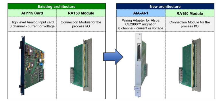
The existing architecture consists of an AH115 card connected to an RA150 on which the process I/O are wired.
