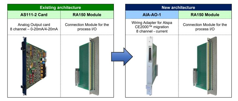
The existing architecture consists of an AS111-2 card connected to an RA150 on which the process I/O are wired.
