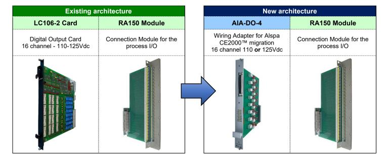
The existing architecture consists of an LC106-2 card connected to an RA150 on which the process I/O are wired.
