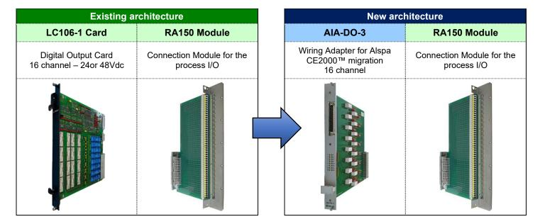
The existing architecture consists of an LC106-1 card connected to an RA150 on which the process I/O are wired.
