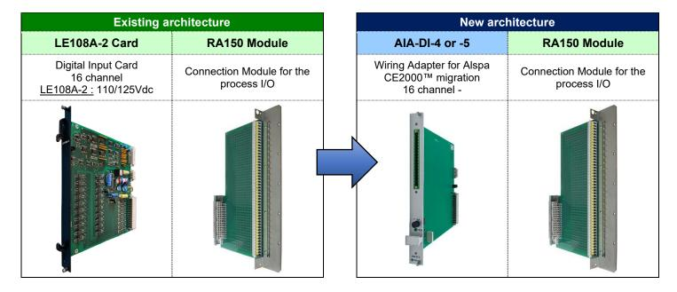
The existing architecture consists of an LE108A-2 card connected to an RA150 on which the process I/O are wired.
