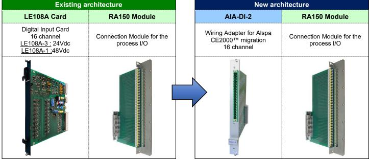
The existing architecture consists of an LE108A card connected to an RA150 on which the process I/O are wired.
